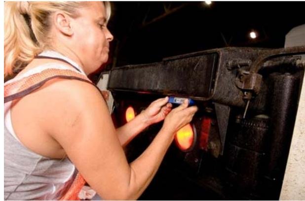
Once tags are fixed, truckers access the web portal to enter their tag ID numbers and associate these with all of their truck ID numbers. This provides a permanent, unique record for each truck, which is used along with bill of lading or container number to pre-advise individual gate moves.
