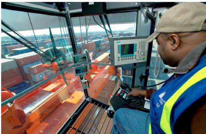
to the data terminal in the RTG operator's cab, where they are automatically 'promoted' to the top of the job list. As containers are stored in the stack, their final location is updated in the PDS system for later use.
